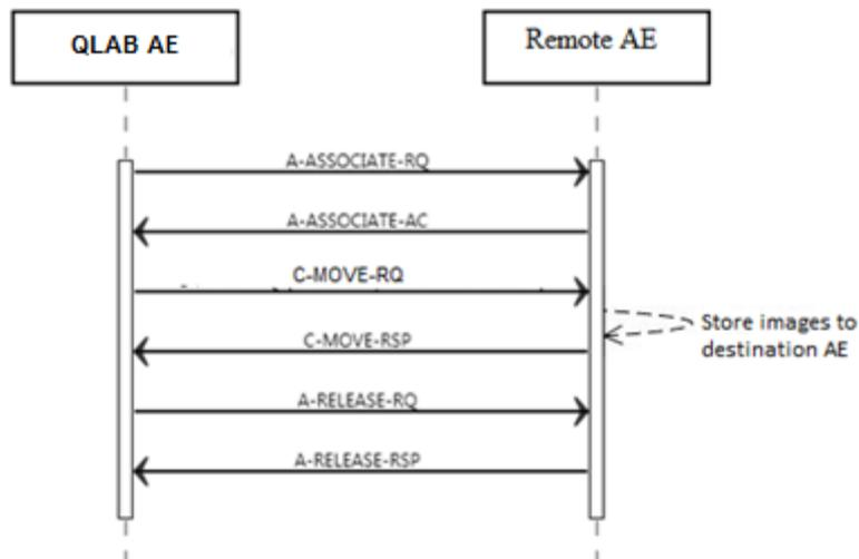
Figure 6 Data Flow Diagram – MOVE as SCU
