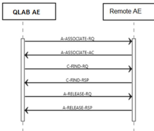
**Figure 5 Data Flow Diagram – FIND as SCU**
